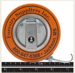
Figure 1.1 Diameter tape used for the inventory
